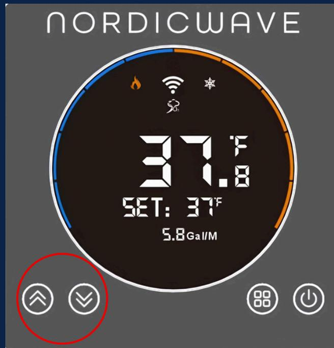
2. Press and hold the "SET" button on the chiller for 6 seconds until you hear a beep. If the connection has been successfully established, the Wi-Fi icon shown in the image will start flashing.
