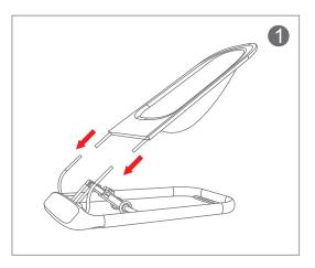
1. Put the connecting elements of the frame into the bouncer base (fig. 1). Make sure they are inserted properly.
