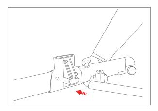
1. Insert the transverse supporting tube into the plastic joint until you hear a clicking sound.
