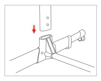
2. Insert the Bracket tube into the plastic joint until you hear a clicking sound.
