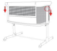
Lift up the plastic height adjust handle both sides, then pull down the nest, it comes lower as you need.
