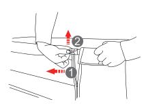
Push the button as indicated by the arrow on the button, then upwards the top rail.
