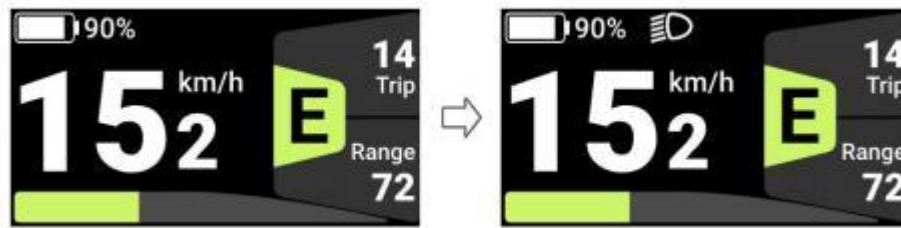
Headlight Switch Interface
