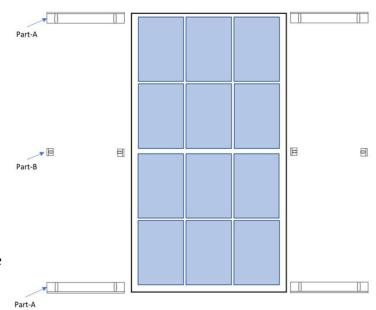
6) Place shutter onto lip of bracket and push back as far as possible. Mark shutter(s) to pre-drill pilot holes into shutter from top & bottom of mounting brackets. Use a 5/32" bit for this step. Insert 1" screws through bracket and into shutter. Tighten screws snuggly – be careful to not over-tighten.
