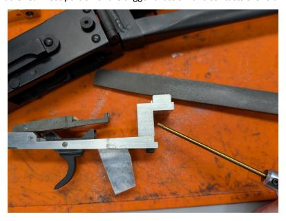
3. Test fit and continue filing the same area until the gap has been eliminated.
