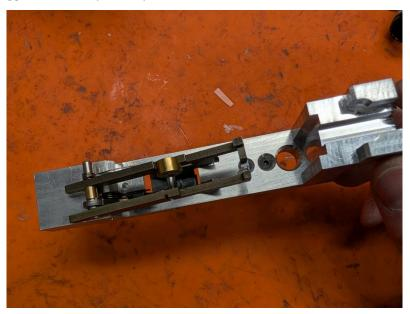
2. Place the trigger chassis into your receiver, ensuring that you keep it flat against the bottom while pushing it backwards
