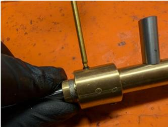
4. Pull the inner barrel forwards out of the chamber
