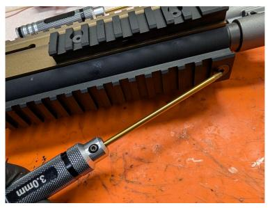
3. Remove the chamber supports from both sides of the upper using the 2.5mm hex wrench and the gas block Torx wrench
