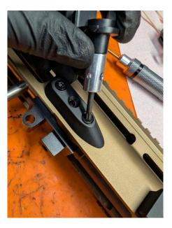
4. Loosen, but do not remove, the bolts on the remaining handguard rail segments using the 2.5mm wrench and Torx wrench
