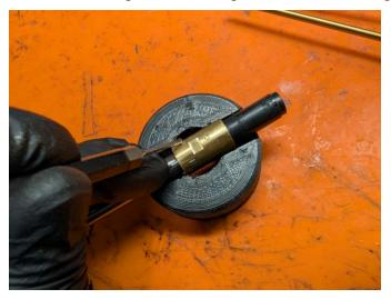
6. Slide the barrel ring forwards off the barrel
