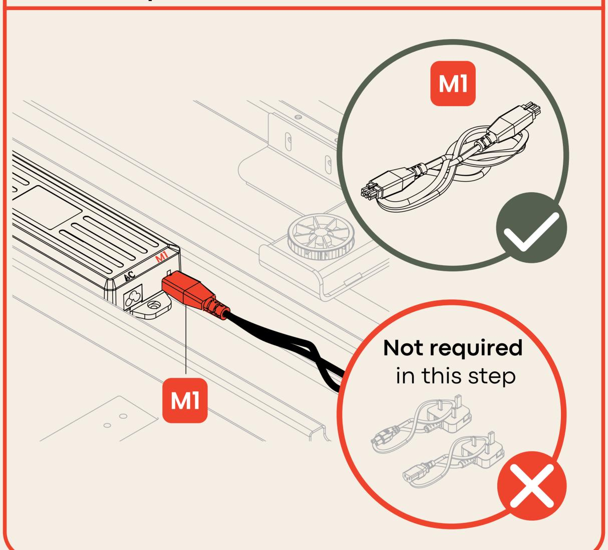
Connect the other end of the Extension Cable with M1 label to M1 port in Desk Base Column with Left label.
