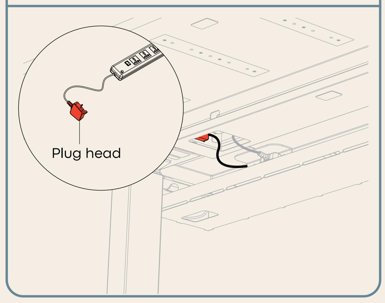
Attach Main Power Cord with M3 label into M3 port located on the Desk Base Column with Left label.
