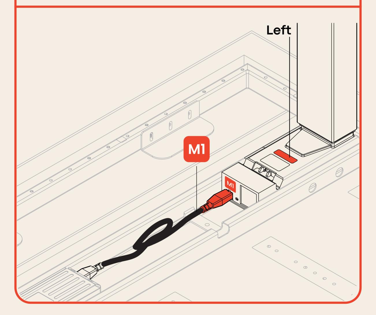
Install Control box Power Cable with AC label to AC port.
