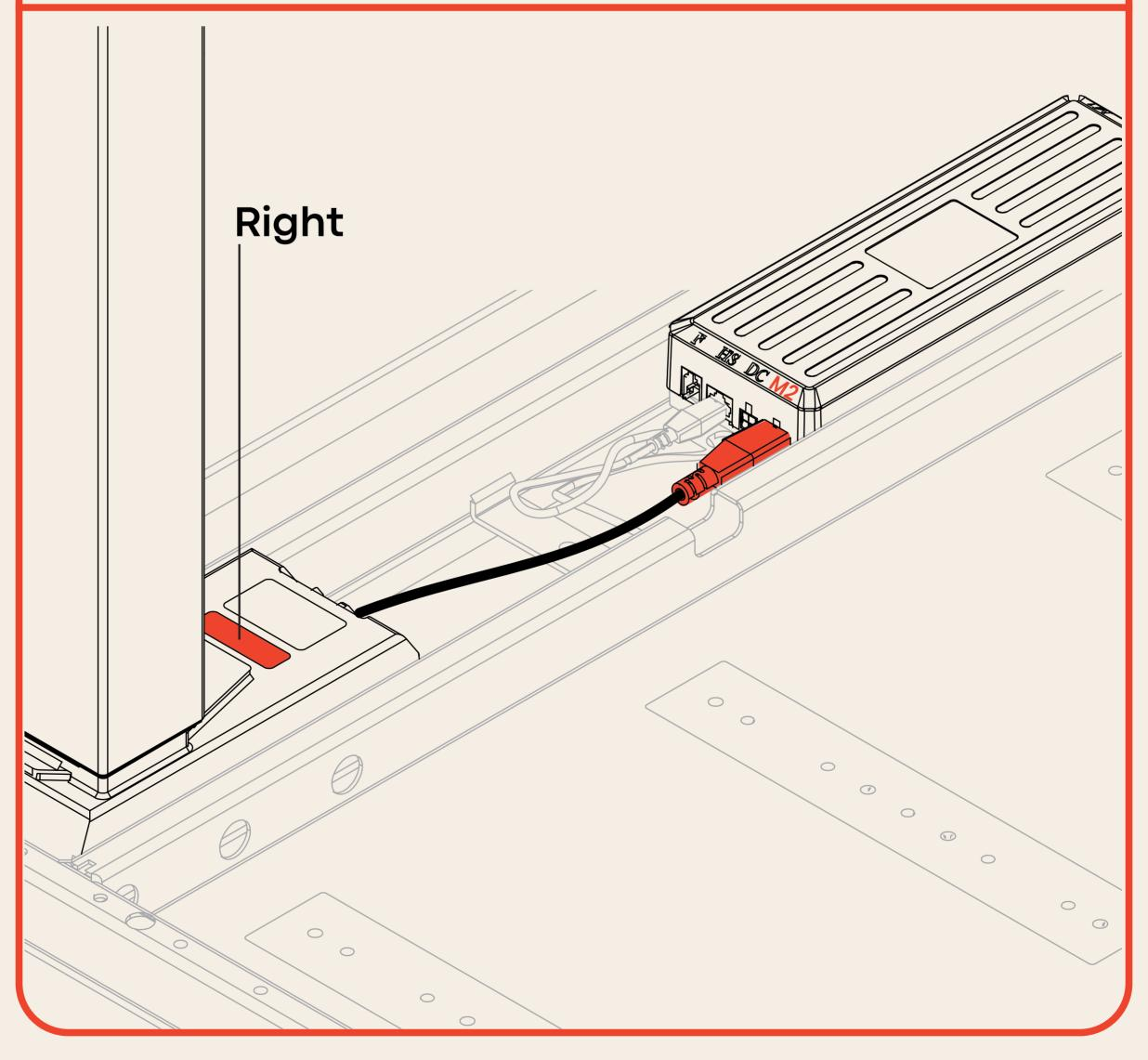
Connect Extension Cable with M1 label to M1 port in Control Box.
