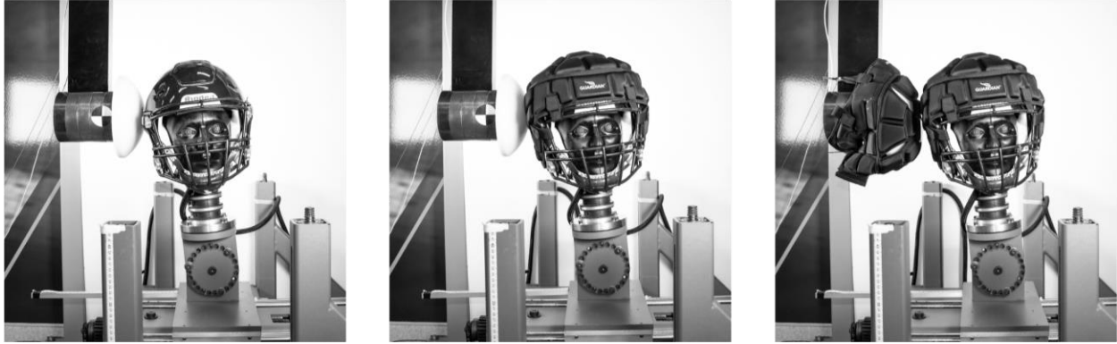
Figure 3. Photographs of shell add-on test configurations from left to right: control, single add-on, and double add-on.
