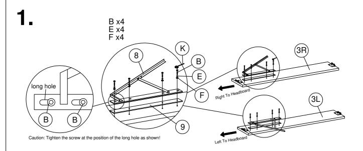
Attach the pump mounting bracket (8) and bracket base (9) to the both side rail (3) using hardware parts B , E , F and K.
