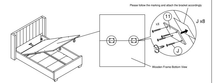
Attach the wooden frame bracket (11) to the wooden frame using hardware parts J and a screwdriver (not provided).
