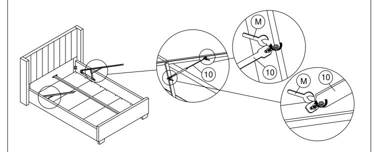
Unscrew the Pre-attached hex-nut of gas spring (10) and attach it back again as shown. Please fully tighten the nut.
