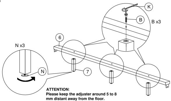
Attach the support legs (7) to the centre rail (6) using hardware parts B and K.
