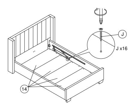
Insert the bottom panel (14) to the below frame and secure using hardware part J and a screwdriver (not provided).
