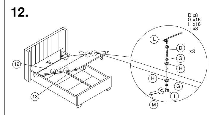
Assembly the wooden frame (12) and wooden frame (13) to the bracket and tighten all the fitting accordingly.
