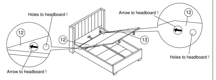
Must place the wooden frame (12 & 13) in correct position (please follow the position as shown in diagram).
