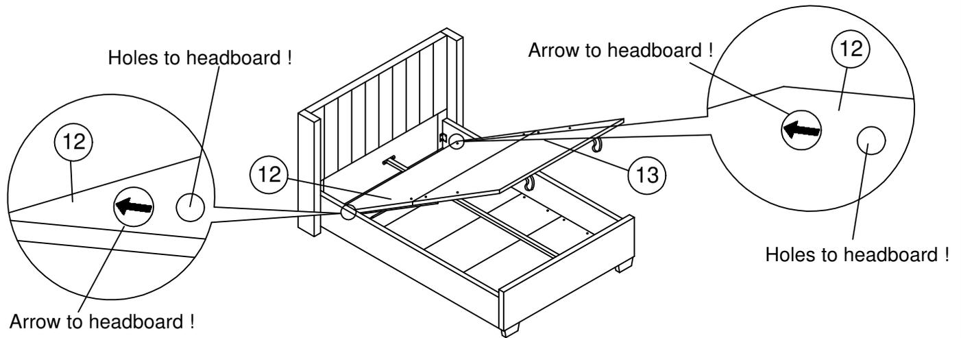
Must place the wooden frame (12 & 13) in correct position (please follow the position as shown in diagram).
