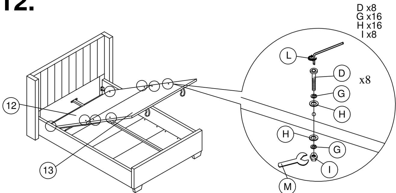
Assembly the wooden frame (12) and wooden frame (13) to the bracket and tighten all the fitting accordingly.
