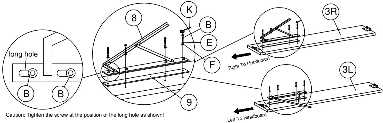
Attach the pump mounting bracket (8) and bracket base (9) to the both side rail (3) using hardware parts B , E , F and K.
