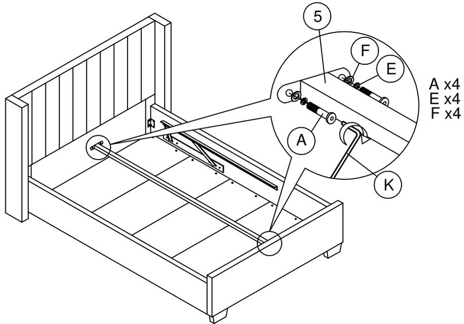
Insert the centre rail (5) to the headend (1) and footend (2) and secure using hardware part A and K.
