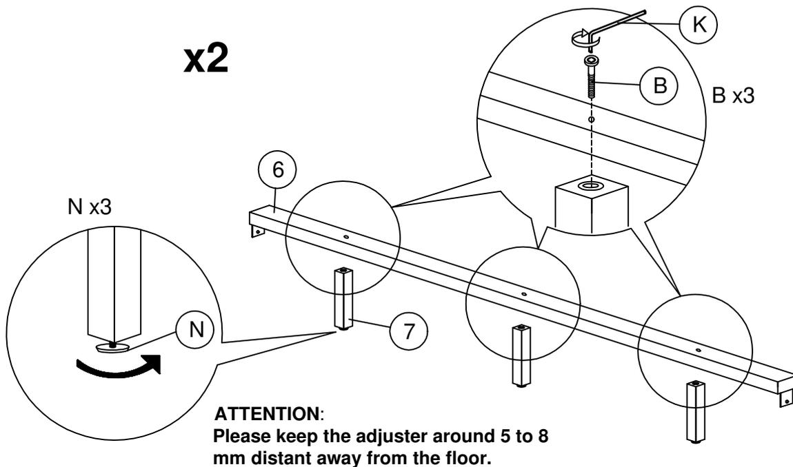
Attach the support legs (7) to the centre rail (6) using hardware parts B and K.
