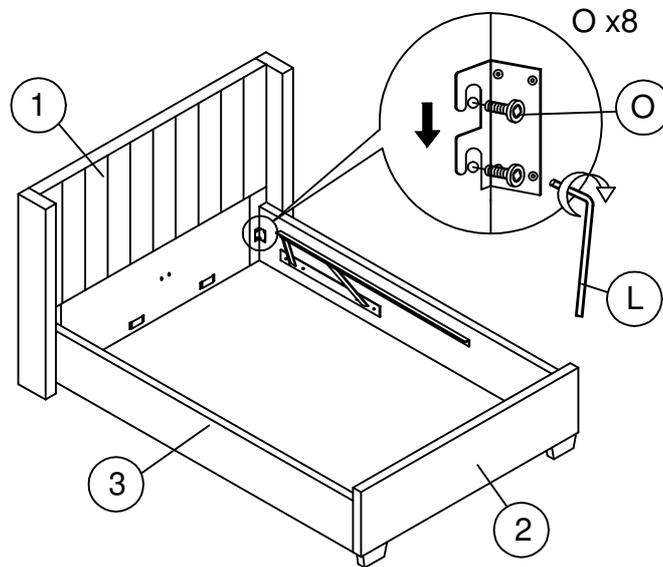
Attach the side rails (3) by pushing the brackets down into place and secure the bolts using hardware part L as shown.
