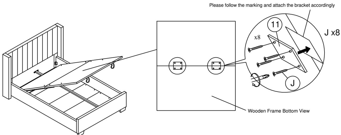
Attach the wooden frame bracket (11) to the wooden frame using hardware parts J and a screwdriver (not provided).
