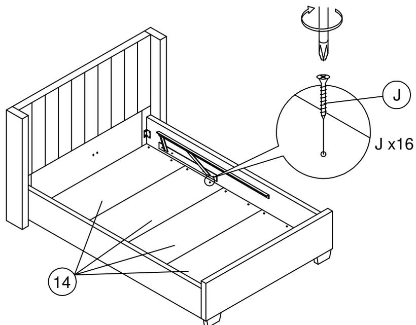
Insert the bottom panel (14) to the below frame and secure using hardware part J and a screwdriver (not provided).
