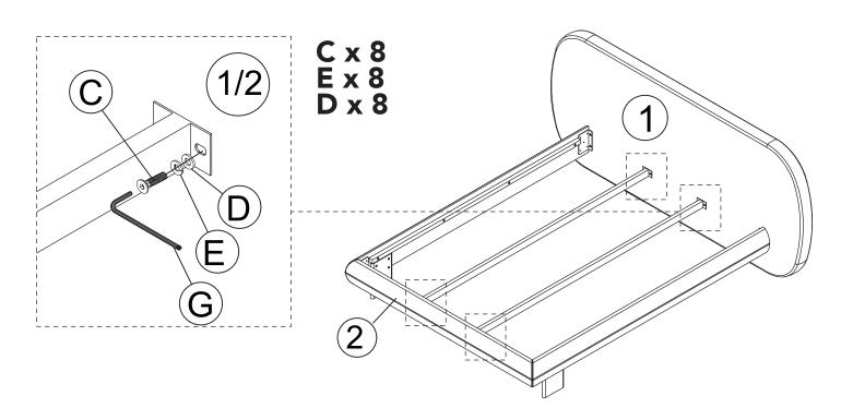
Connect Footboard (2) to Siderail Left & Right (3/4), use JCBB M8 x 30mm (A), screw in with Allen Key M5 (H). Install Metal Center Rails (5) between the headboard and footboard, use JCBC M6 x 25mm (C), Spring Washer M6 x 12mm (E) and Flat Washer M6 x 19mm (D), screw in with Alley Key M4 (G).
