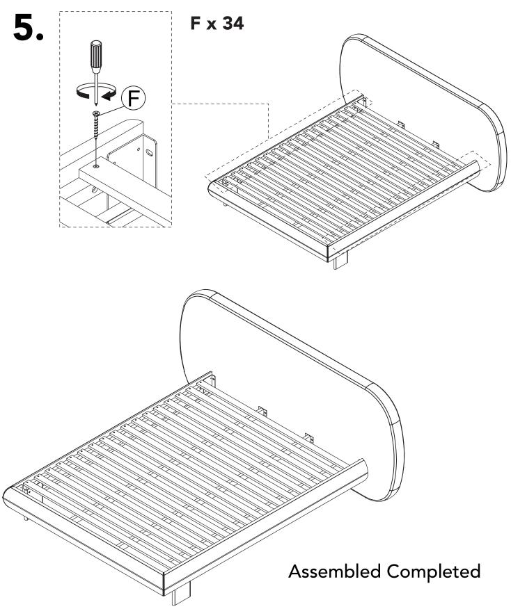
Place the Slats (4) on the bed frame. Secure each slat with CSK M4 x 38mm (F). Reminder: Please ensure all bolts and screw are tightened and secure before you use it.
