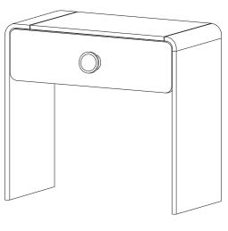
Take out the Handle (2) from drawer. Tigthen the Handle(2) with Screw M4 x40mm
