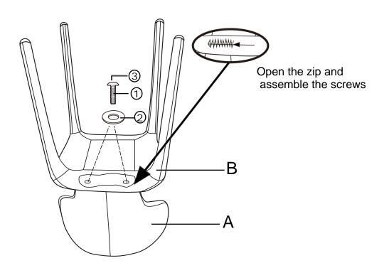
Insert the backrest(Part A) into the seat(Part B). Open the zip which under the seat  $\,$ , put the gasket (Part  $\,$ ) on the hole ,use allen key ( Part  $\,$ ) assemble the screws(Part  $\,$ )
