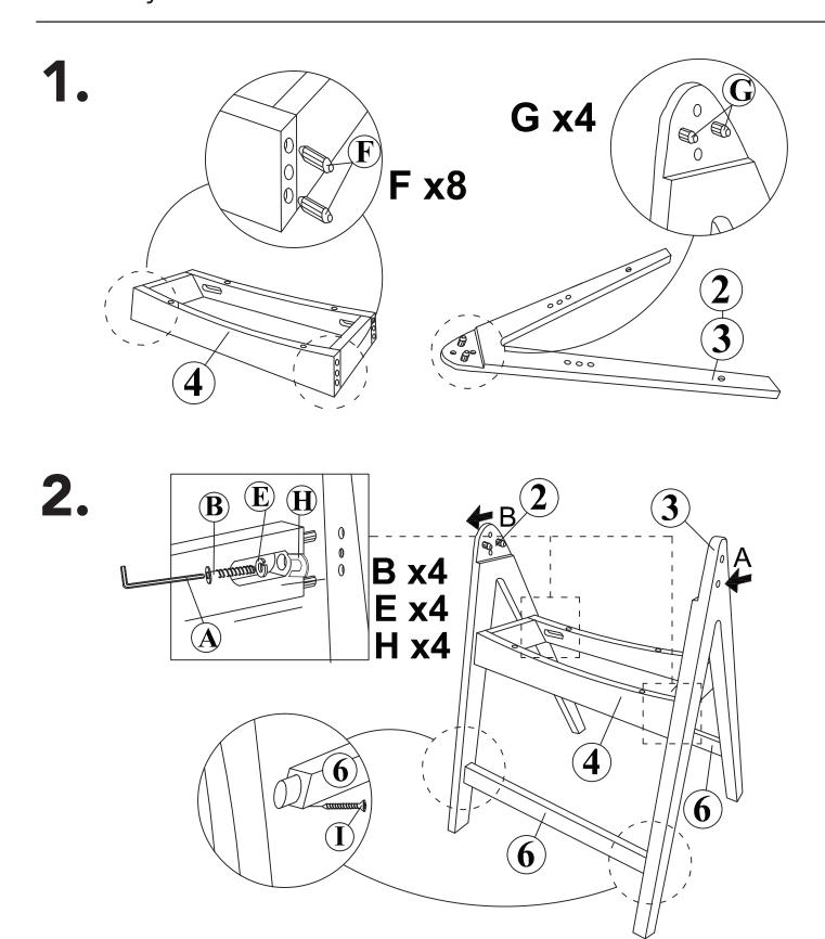
Place a washer (**Part E**) on a bolt (**Part B**), and insert it into the hole of the Apron (**Part 4**) as pictured, (there will be 4 of these per chair), use the long end of the tool (**Part A**), to screw the bolt (**Part B**) halfway into the threads preinstalled into Leg A/B (**Parts 2/3**) do not tighten 100% & do not put **washer H** in place yet (this will assist installation of the backrest and footbar in the later steps of this assembly)
