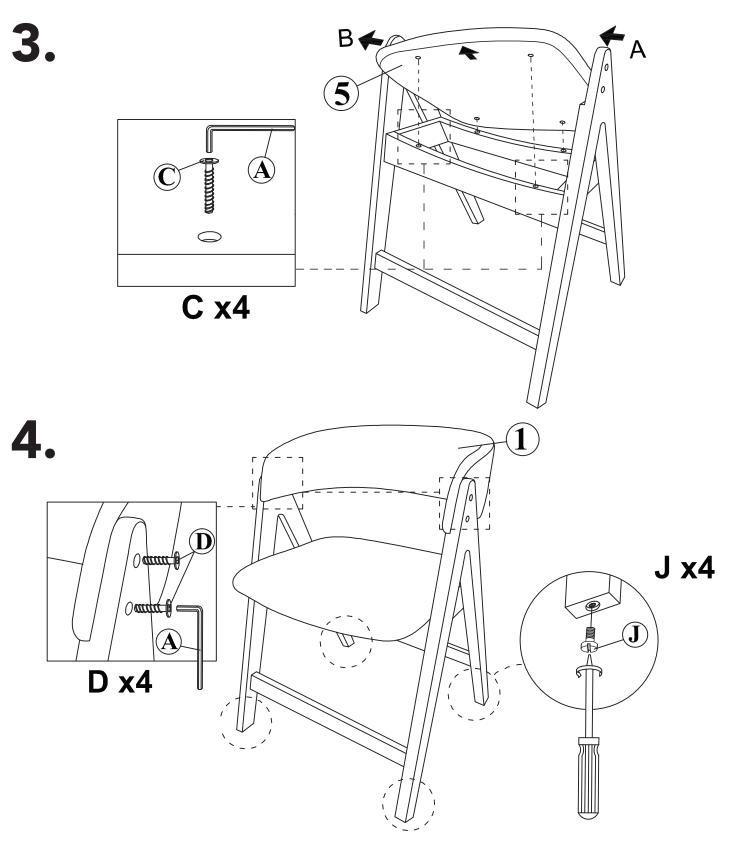
With the Backrest (**Part 1**) and Bolts (**Part D**) screwed in halfway, you should now begin tightening the Bolts (**Part B**) the rest of the way into the apron (**Part 4**) and now is the perfect time to put the H washers in place, once it gets hard to turn you will need to turn the tool (**Part A**) around and use the short end in order to get more leverage and to ensure a complete and satisfactory assembly
