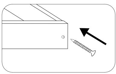
STEP 10 Attach Back Panel to Cabinet Using Pin Head (  $3.5 \times 16$  )
