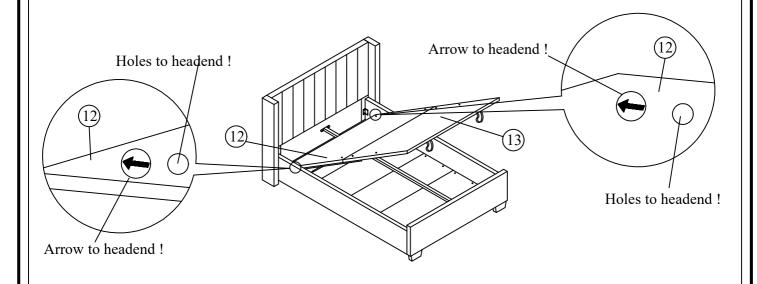
Step 12: Assembly the wooden frame (12) and wooden frame (13) to the bracket and tighten all the fitting accordingly.
