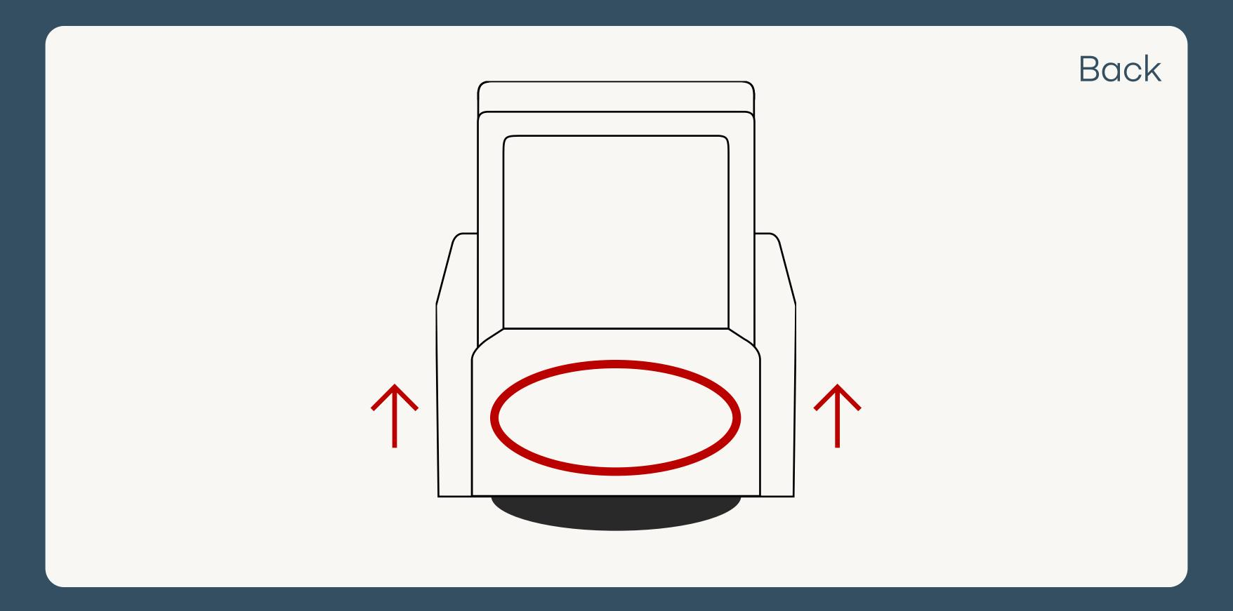
**Step 2:** Pull each clip outwards one side at a time, and then pull the back up. Please be sure to also disconnect the wires.
