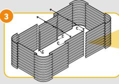
Assemble all side panels first and then attach to the corner sections. Ensure that you attach the corners on the outside of the straight sheets. Bracing channel is installed at this point.
