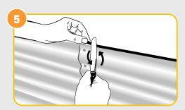
Remove the remaining protective plastic. Starting on a straight length of steel, push the safety edge over the rolled steel edge. Where the steel panels join using a butter knife to pry open will assist in attaching. **IMPORTANT:** Ensure the safety edge starts and finishes on a straight section of steel, preventing detachment.
