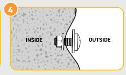
Attach all nuts loosely & then tighten using a screwdriver /cordless drill assists with this process. Failure to tighten each nut and bolt to its maximum may cause failure.
