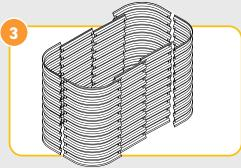
Assemble all side panels first and then attach to the corner sections. Ensure that you attach the corners on the outside of the straight sheets.
