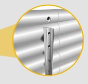
**NOTE:** Channel is installed at this point, see configuration diagrams marked in C for their locations. Affix 2 lowest bolts only.
