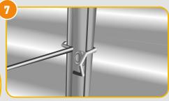
Note where the brace rests on top of the corrugation. Affix 3 remaining bolts above each channel.
