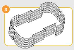
Assemble all side panels first and then attach to the corner sections. Ensure that you attach the corners on the outside of the straight sheets.
