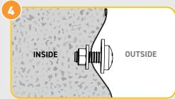
Attach all nuts loosely & then tighten using a screwdriver /cordless drill assists with this process. Failure to tighten each nut and bolt to its maximum may cause failure.
