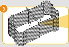
Assemble all side panels first and then attach to the corner sections. Ensure that you attach the corners on the outside of the straight sheets. Bracing channel is installed at this point.
