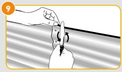
Remove the remaining protective plastic. Starting on a straight length of steel, push the safety edge over the rolled steel edge. Where the steel panels join using a butter knife to pry open will assist in attaching. **IMPORTANT:** Ensure the safety edge starts and finishes on a straight section of steel, preventing detachment.
