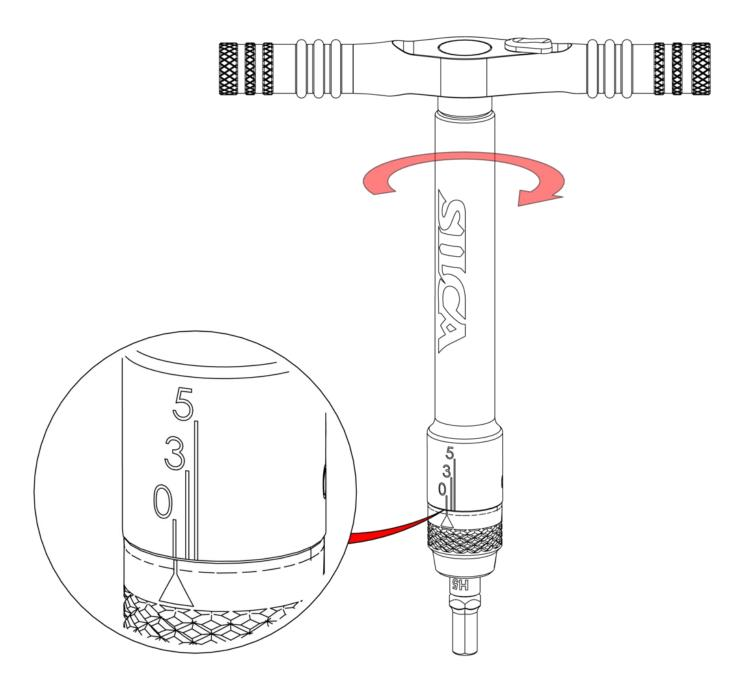
With the 1/4" drive bit engaged, begin to tighten the bolt.
