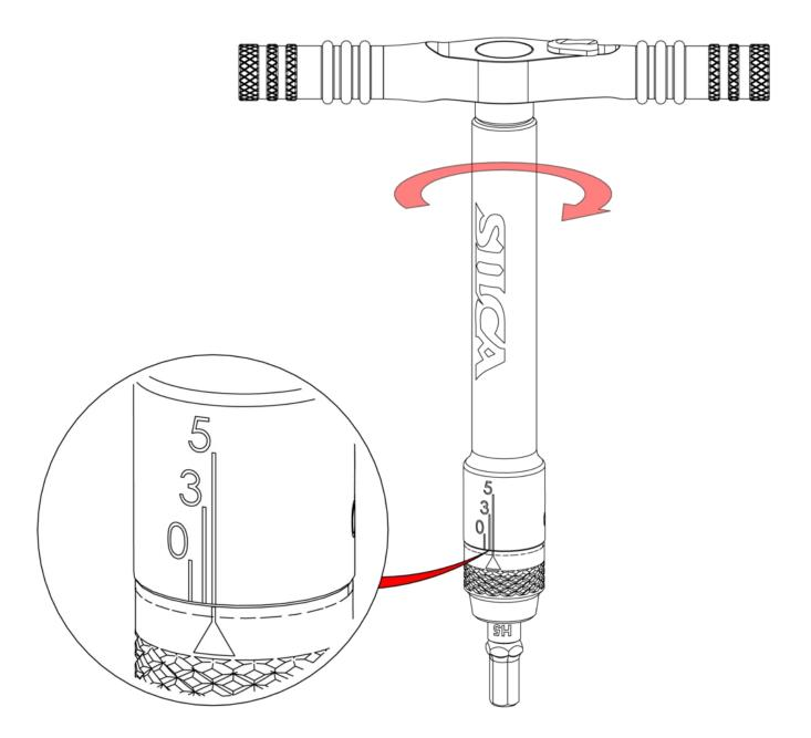
During the process of tightening the bolt, do not exceed the maximum intended torque specification.
