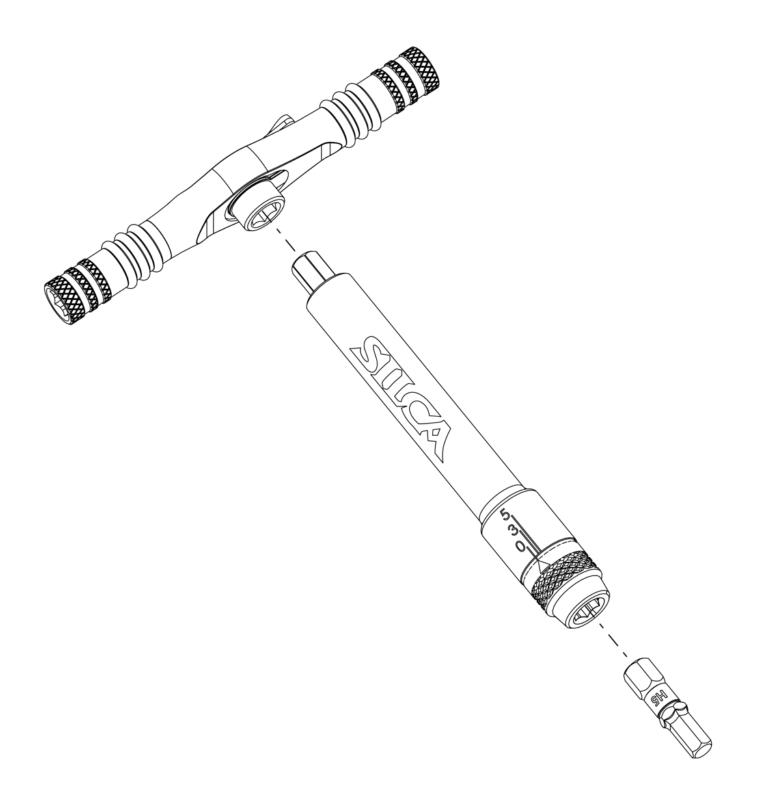
Insert Ti-Torque into T-Ratcher or similar 1/4" drive tool.
