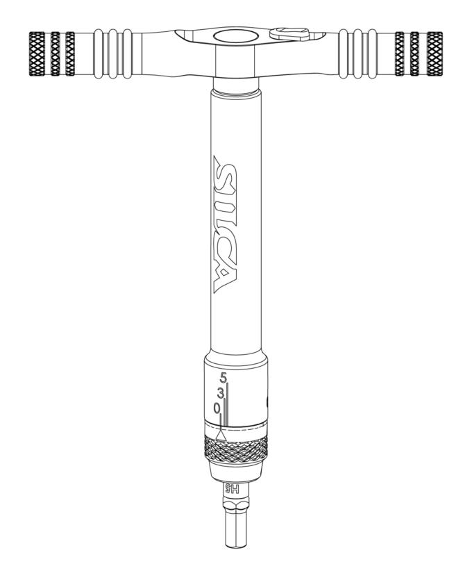
Each scale view shows a zero [0] mark indicating the calibrated resting spot.
