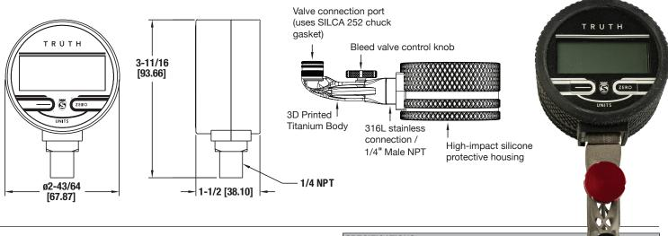
The TRUTH Digital Pressure Gauge has a precise  $\pm 1.0\%$  full scale accuracy. The four digit digital display will reduce the potential for errors in readings by eliminating parallax errorr commonly produced with analog gauges.
