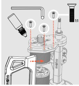
Using the 1/8 hex key, fit the Protection Bars onto the Left Plate with 3 x 14mm bolts (5).
