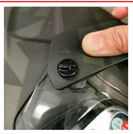
1. Align shield and visor with the pivot hole as shown, then install the screw. Do the same procedure on both sides.
