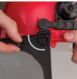
**5.** Choose the visor you wish to attach and fasten it to the visor support by aligning the slots on top of the visor with the locking system. Turn the black knobs to lock the visor into place. Make sure the visor can be raised and lowered freely and is securely locked in place.
