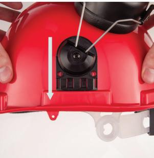
**3.** Attach the ear muffs by sliding their connectors into the top of the cap slots on each side of the helmet until they click into place. Each ear muff can be attached to either side. Rotate and place the ear muffs in their resting position on the back side of the helmet to allow for easy further assembly.
