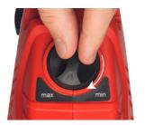
For thicker paints (more than 50 DIN/s) - turn the dial clockwise to maximum for when you need to quickly cover a large area.
