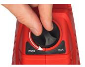
For thinner paints (less than 50 DIN/s) - turn the dial anti-clockwise to minimum for when you need a more steady, deliberate spray.
