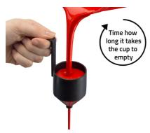
Place your finger over the hole of the included flow cup and fill it to the brim with your chosen material. At the same time, release your finger from the hole, and start the timer. Stop the clock when the flow cup has completely drained of paint.
