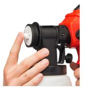
4. Insert your new nozzle tip and make sure it fits nice and snug. Screw the nozzle cap back on tight.
