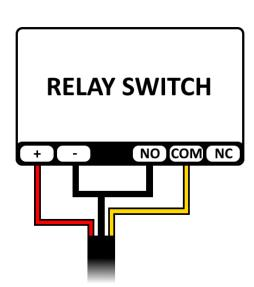
Illustrates the wiring for a typical momentary relay switch. In this case, the relay switch is powered by the AutoSlide system and not a separate power supply.
